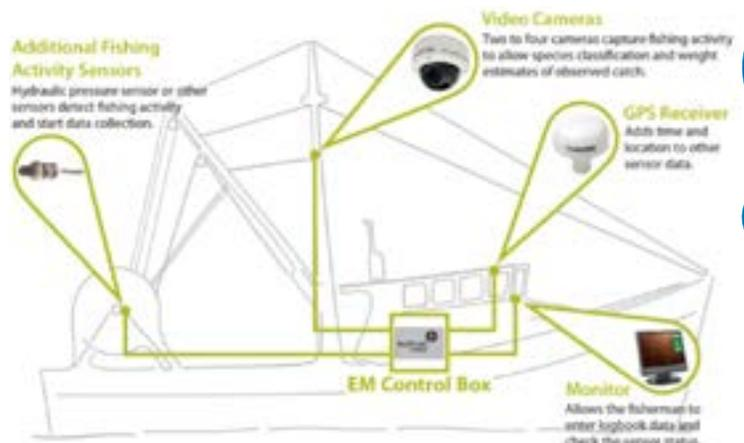
Figure 1. Diagram of an electronic monitoring system on a gillnet fishing vessel. Source: Ecotrust Canada.
