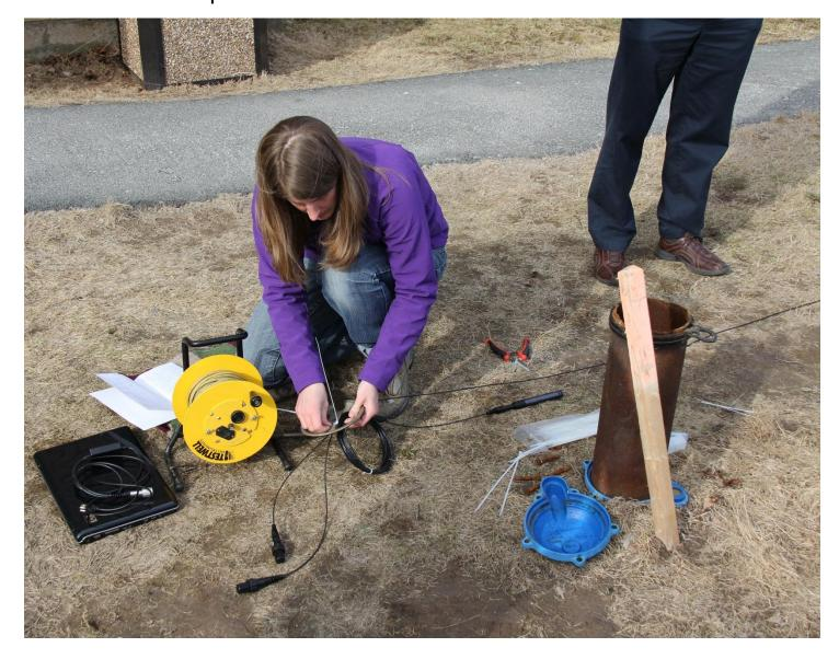
Note here you can see the levelogger cord length is quite long and goes off the page (around 10 m). The barologger cord is quite short, around 1 m. The levelogger must be suspended into the water when it is installed and the barologger must stay above the water level.
