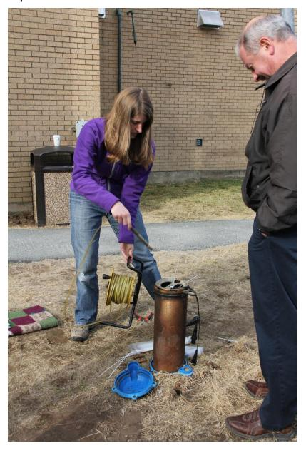
After this step, also assess the depth of the well. Turn off the WLR probe, and continue to lower the device into the well by unrolling the spool. Do not unroll it too quickly as it could smash at the bottom of the well (or meet and obstruction) or damage the probe(s). Record the depth of the well and/or the depth of any obstructions. It is also possible that the well is deeper than the spool, in which case historic data (such as drilling logs) will suffice for this information.
